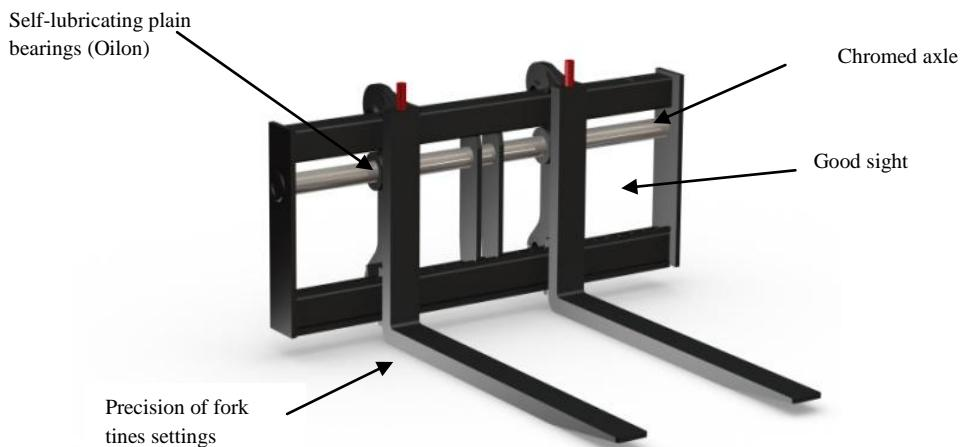
**ABL CE**, can in this range as standard offer mechanical pallet forks from **2,5tons** to **20 tons**. Frame width between **1000mm** to **2500mm**. Attachment connection. The fork tines are **1200, 1400, 1500** and **1600mm** as standard. The pallet fork's capacity is by tp. 600mm.
