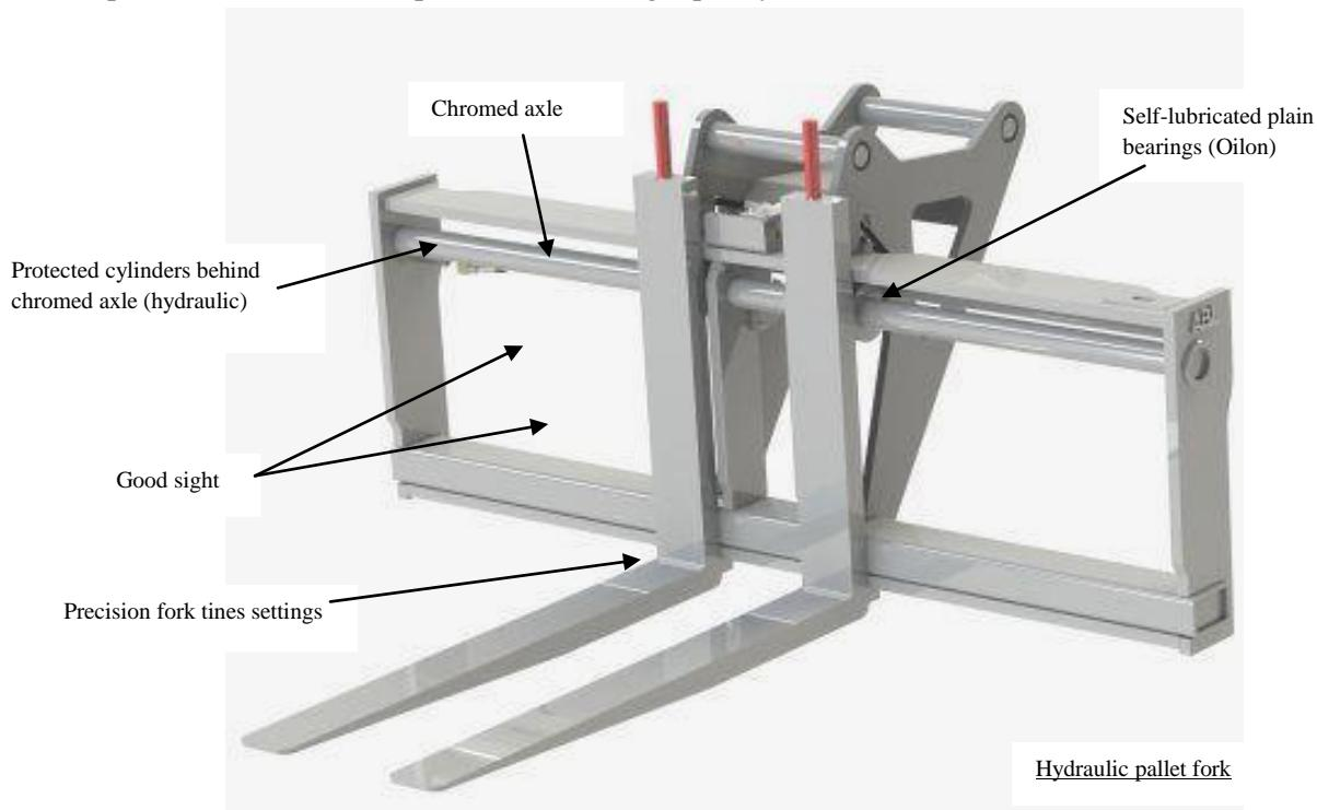
**ABL CE** can in this range as standard offer mechanical pallet fork from **1.0tons** to **5.0tons** and a frame width **1000mm** to **1500mm**. The length of the fork tines are **1200mm** as standard. Depending on sizes there are attachments for quick couplers S40-S70 or S1-S3. The pallet fork's capacity is by tp. 600mm.
