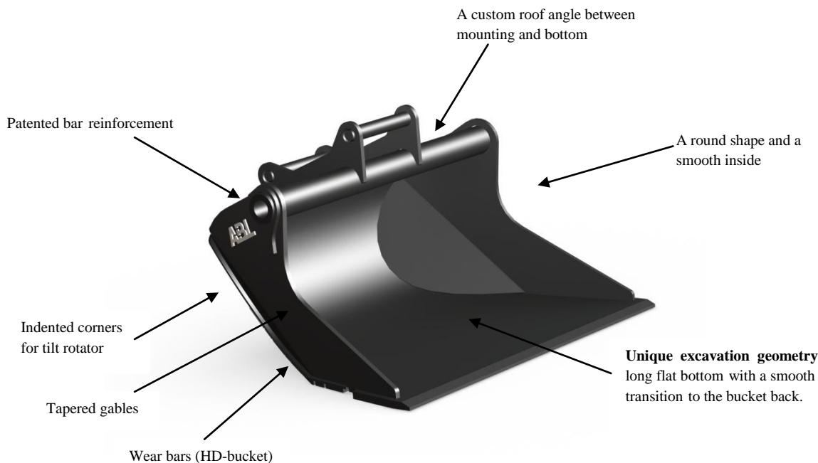
**ABL CE**, can in this range as standard offer grading buckets from **40L** to **2200L**. Widths between **700mm** to **2200mm**. Grading buckets are available as HD and LT version.
