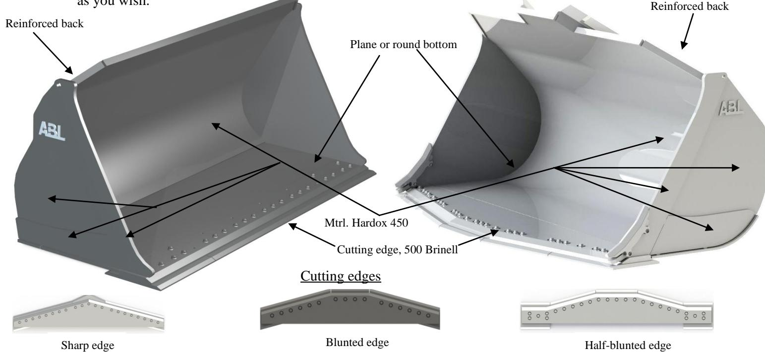
**ABL CE**, can in this range as standard offer different sizes from **1000L/2000mm** to **10000L/3800mm**. Equipped with Volvo or CAT base cut and a connection for a quick coupler.
